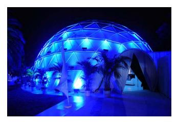
The Vortex Dome is planned for installation in June, 2010, and is a 50' diameter, 150-seat geodesic dome fastened to the outdoor patio on the Beaudry Building. The dome will be fitted with removable seating, a medium-resolution single-projector fulldome display and stereo audio system suitable for public presentations. It is equipped with an internal negative pressure projection screen with low reflectance for maximum image contrast.
